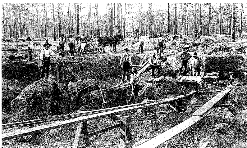
Soil without phosphorus is barren. Here, workers in Florida around 1890 mine phosphoric acid, which is used to make fertilizer.
